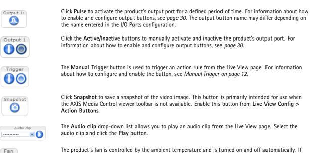
required, the fan can be activated manually by clicking the Fan button. To show the button, go to Setup > Live View Config. Under Action Buttons, select Show fan button and specify the number of minutes the fan should be activated.
