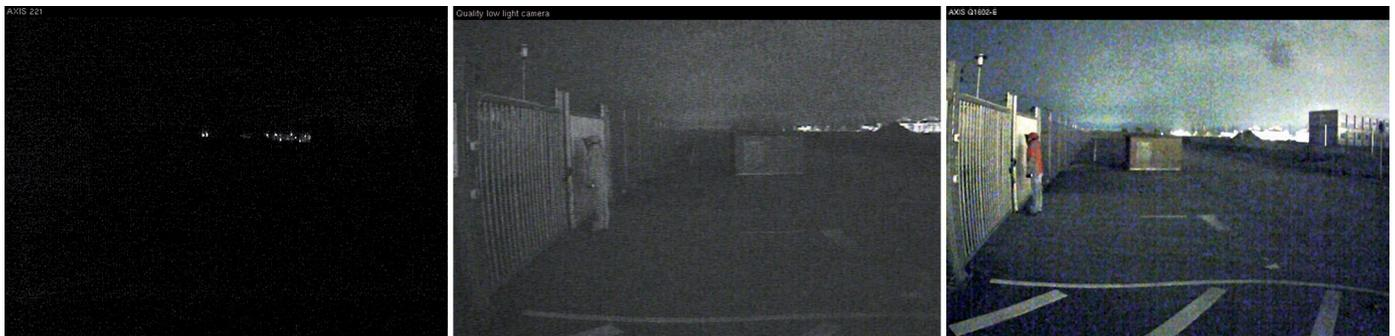
Lightfinder technology with AXIS Q1602/-E, AXIS Q1614/-E Network Cameras
